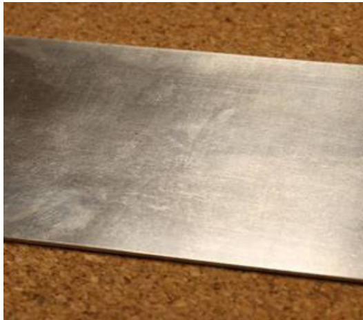
Fig. 3. Stripped steel after mechanical cleaning and degreasing
